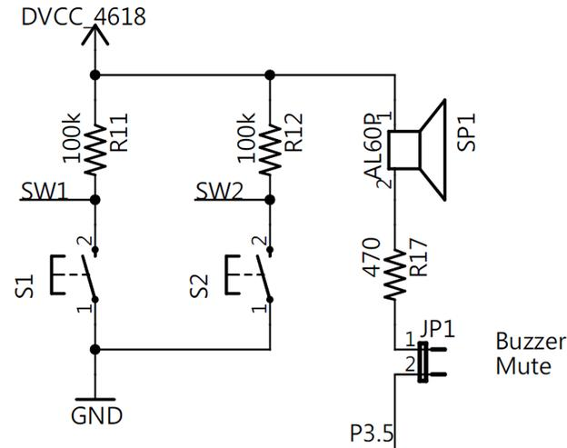
**Figure 4. MSP430 Experimenter Board Switch Schematic**
