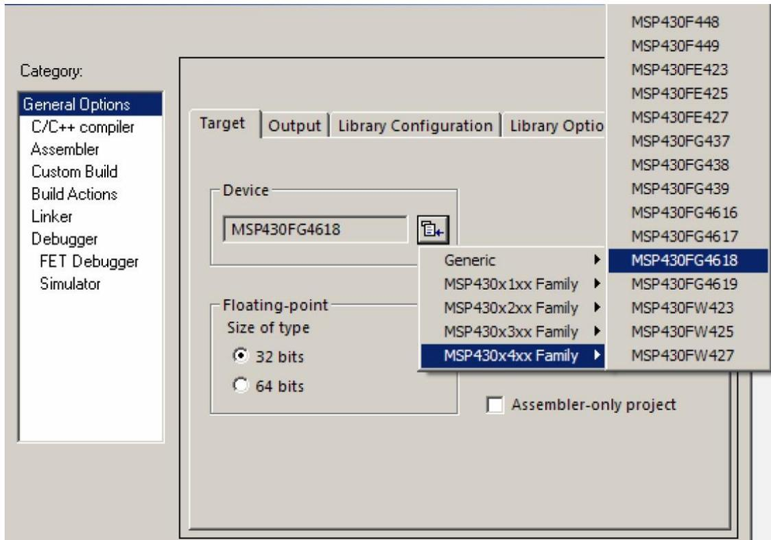
Figure 6. Specifying device (MSP430FG4618) in IAR Workbench.
