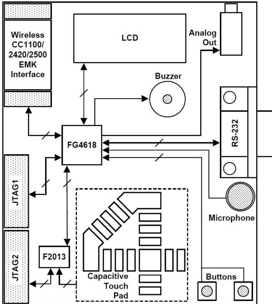
Figure 2. Block Diagram of the Experimenter's Board.
