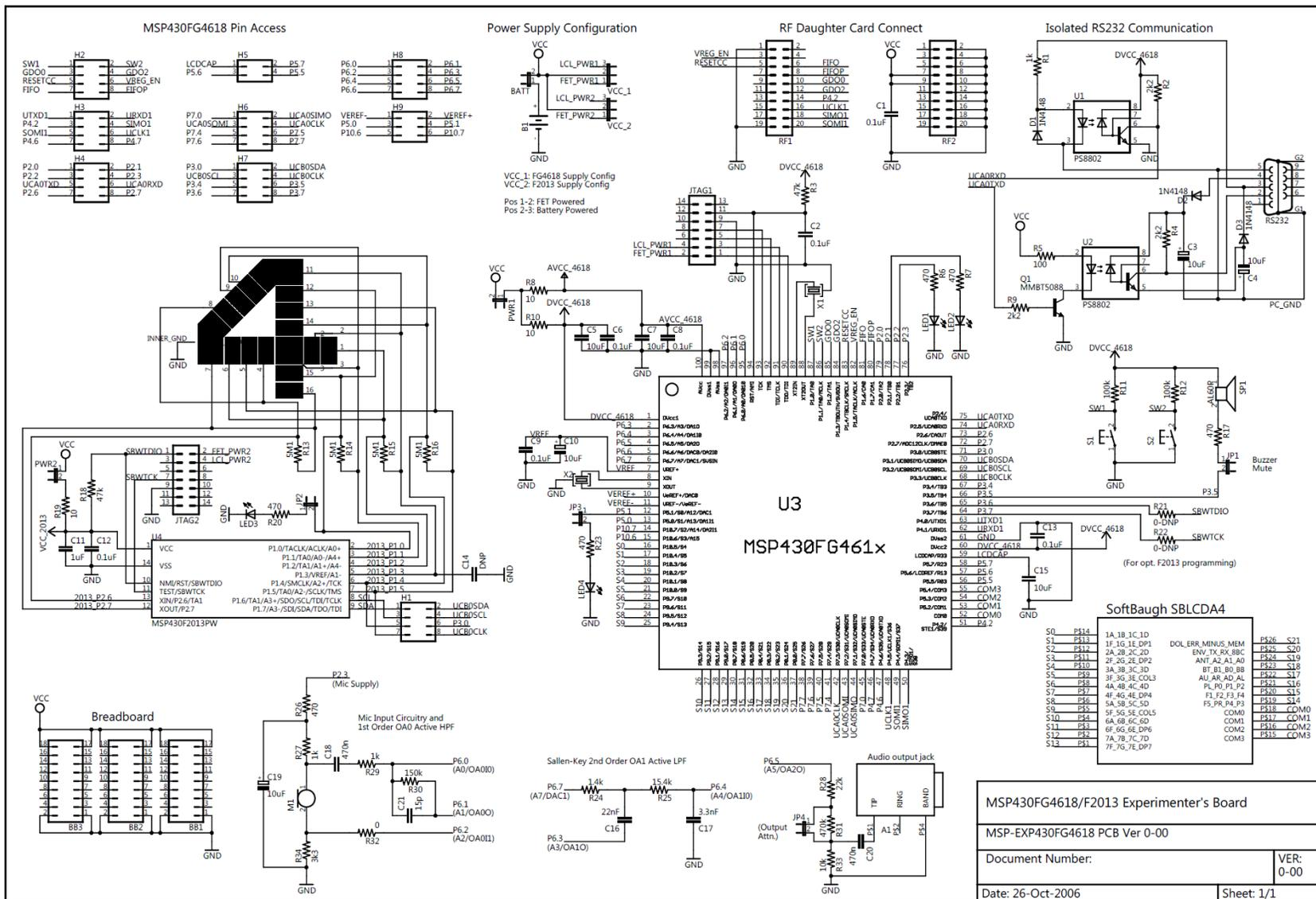
Figure 8. Experimenter's Board Schematic
