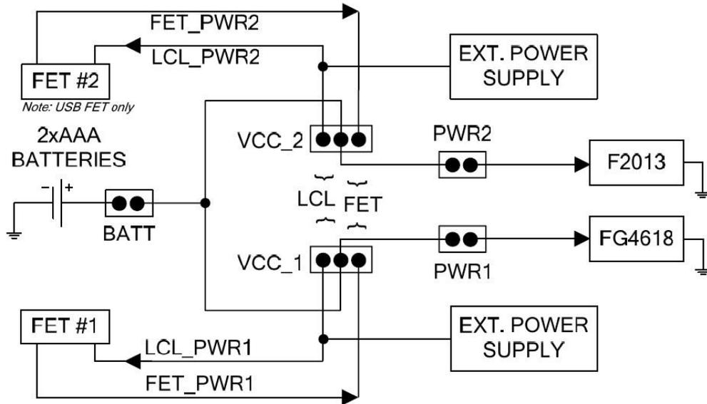
**Figure 3. Board Power Supply Configuration.**
